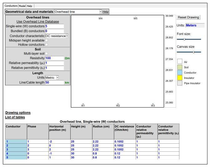
Figure 3 Line/Cable Data device input for modeling the three-phase line of Figure 2.
