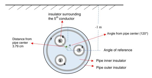
Figure 11 Pipe-type cable example.
