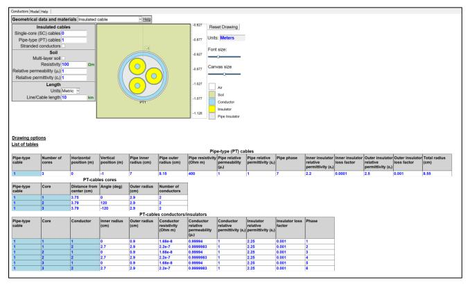
Figure 12 Line/Cable Data device input for the pipe-type cable of Figure 11.
