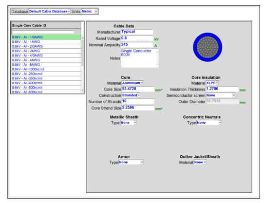
Figure 10 Single-core cable database.
