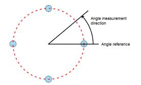
Figure 4 Bundle of 4 conductors, example at 0 degree.
