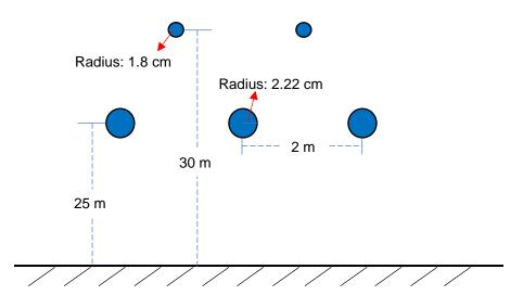
Figure 2 Three-phase overhead line with ground conductors.
