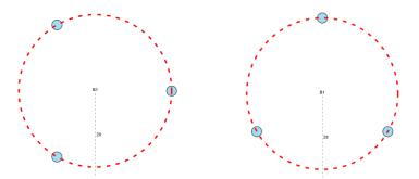
Figure 5 Bundle of 3 conductors at 0 degree (left) and 90 degrees (right).
