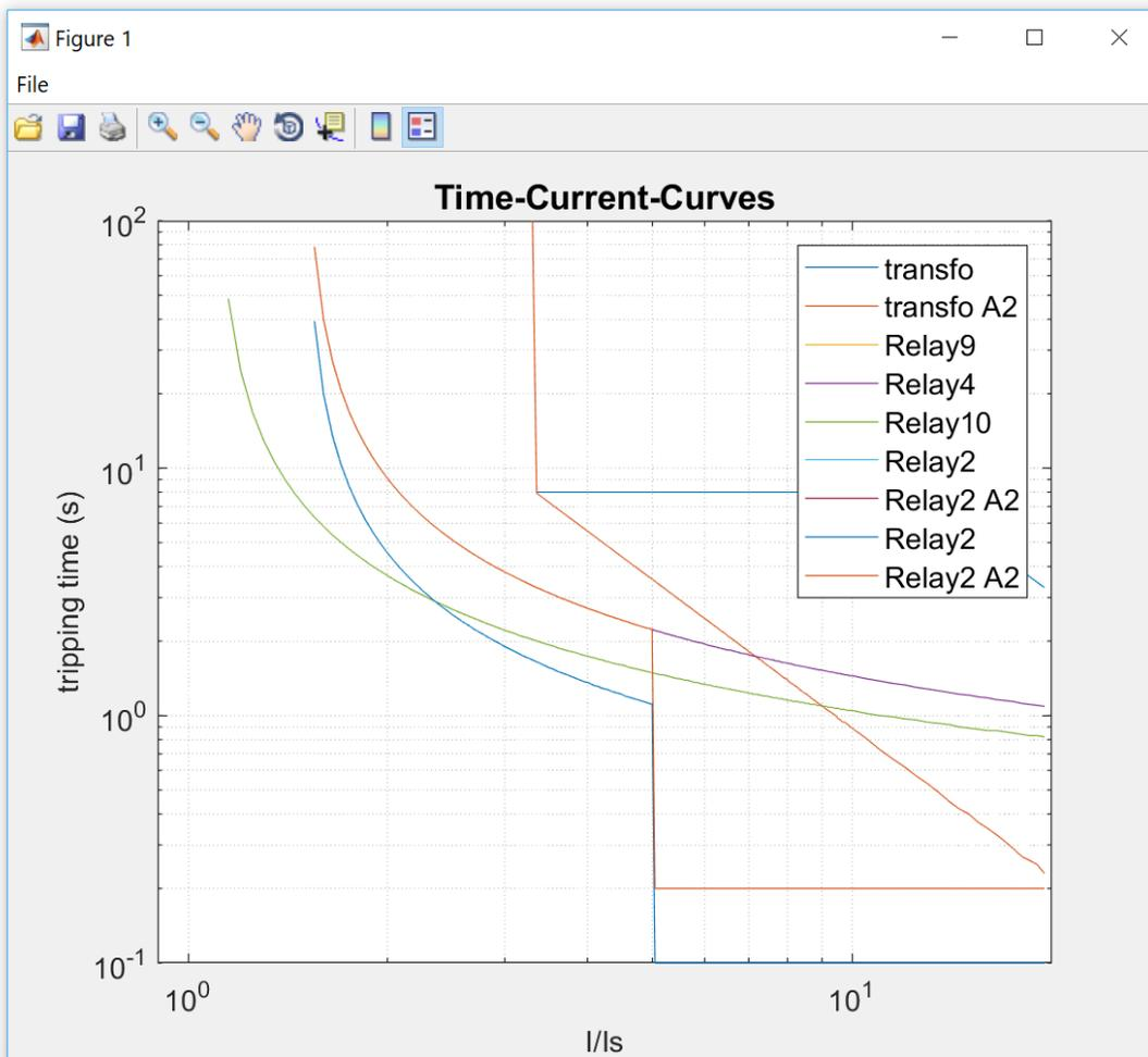
Figure 2-1 Sample time-current graphs for selected signals (coordination curves).
