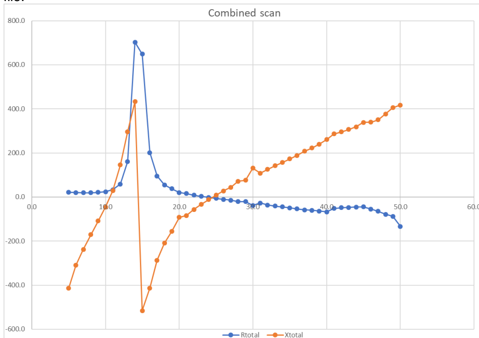
Figure 9 Combined scan: WP impedance added to Grid impedance
