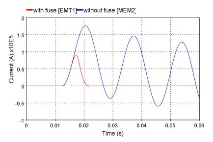
Figure 1-2 Fuse limited short-circuit current and current without fuse
