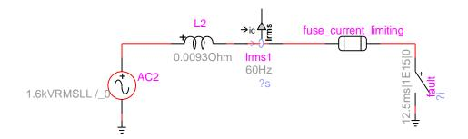
Figure 1-1 Circuit for fuse resistance adjustment (see Toolbox examples folder currentLimitingVSexpulsion.ecf).
