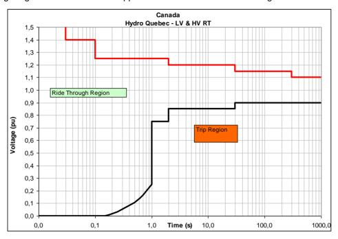
Figure 31 LVRT and HVRT requirements [16]
