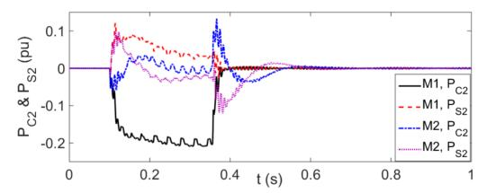
Figure 47 Pc2 and Ps2 of aggregated FSC WT in scenarios M1 and M2
