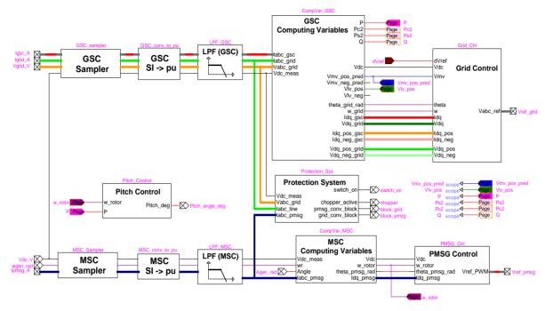
Figure 22 EMTP-RV diagram of FSC "WT Control System" block
