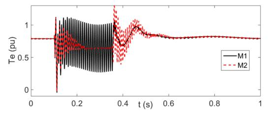
Figure 54 IG electromagnetic torque in scenarios M1 and M2 (with larger size GSC)
