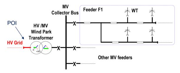
Figure 1 Simplified single-line diagram of a typical wind park
