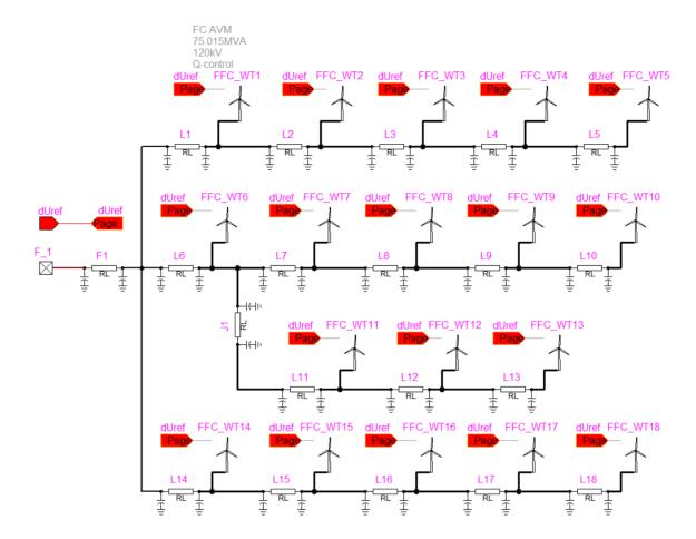
Figure 75 EMTP diagram of MV Feeder-1
