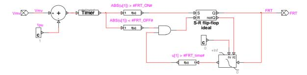
Figure 29 EMTP diagram of "FRT decision logic" block
