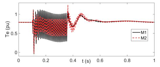
Figure 53 IG electromagnetic torque in scenarios M1 and M2
