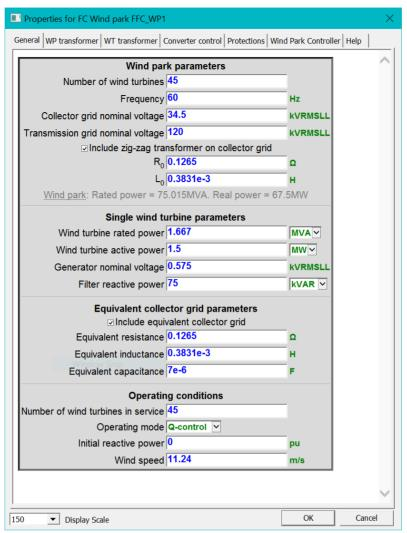
Figure 12 FSC based wind park device mask
