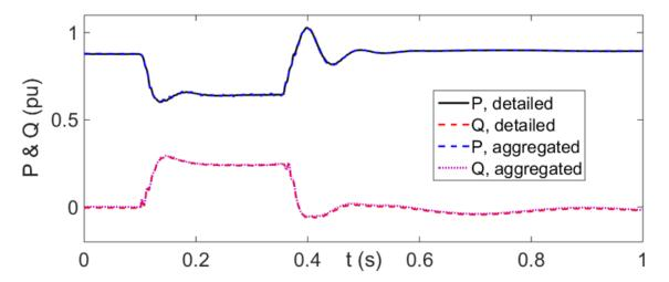
Figure 77 Active and reactive power at POI, Wind Park with FSC WTs
