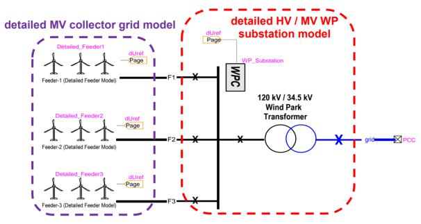
Figure 73 EMTP diagram of the 45 x 1.5 MW wind park detailed model given in Figure 46.
