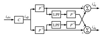
Figure 30 Sequence extraction using decoupling method.
