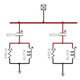
Figure 21 "shunt ac harmonic filter" block
