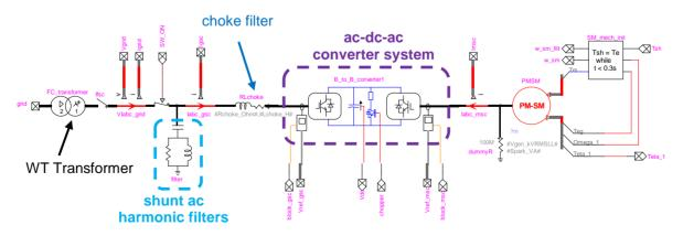
Figure 20 EMTP diagram of FSC "WT Electrical System" block
