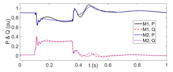
Figure 55 P and Q of aggregated DFIG WT in scenarios M1 and M2
