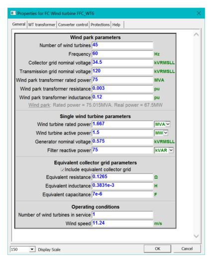
Figure 76 Aggregated FSC based wind turbine device mask
