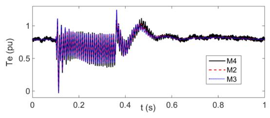
Figure 63 IG electromagnetic torque in scenarios in scenarios M2 - M4
