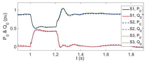
Figure 68 P<sub>0</sub> and Q<sub>0</sub> of aggregated FSC WT in IEEE 39 bus system simulation
