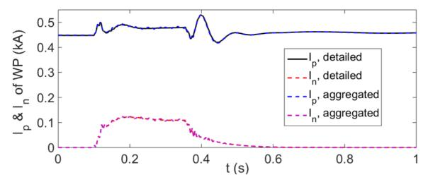
Figure 78 Positive and negative sequence currents at POI, Wind Park with FSC WTs
