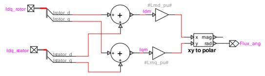
Figure 38 Flux angle calculation
