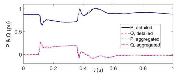
Figure 79 Active and reactive power at POI, Wind Park with DFIG WTs
