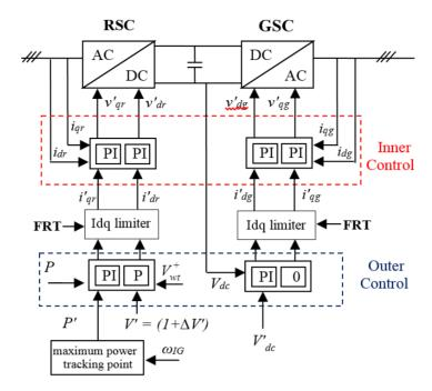
Figure 10 Schematic diagram of DFIG WT control
