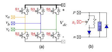
Figure 14 (a) Two-level Converter, (b) IGBT valve
