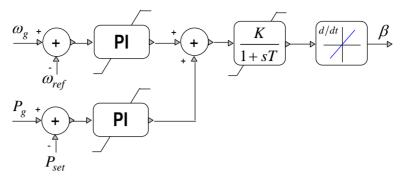
Figure 4 Schematic diagram of pitch control
