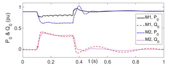
Figure 48  $P_0$  and  $P_0$  of aggregated FSC WT in scenarios M1 and M2
