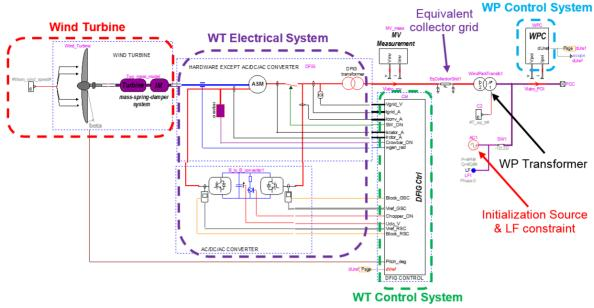
Figure 35 EMTP diagram of the DFIG based Wind Park
