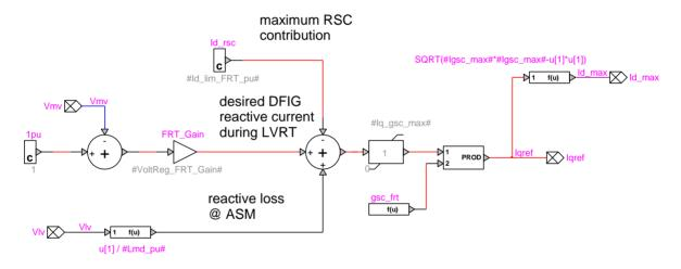
Figure 43 EMTP diagram of "LVRT boost" block
