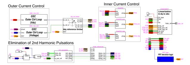
Figure 25 EMTP diagram of FSC "Grid Control" block
