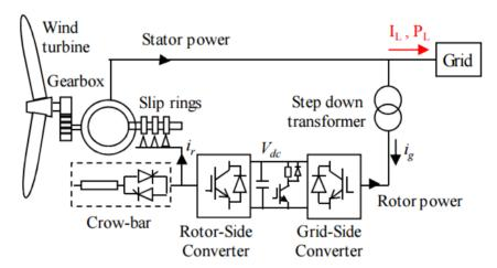
Figure 9 DFIG wind turbine configuration
