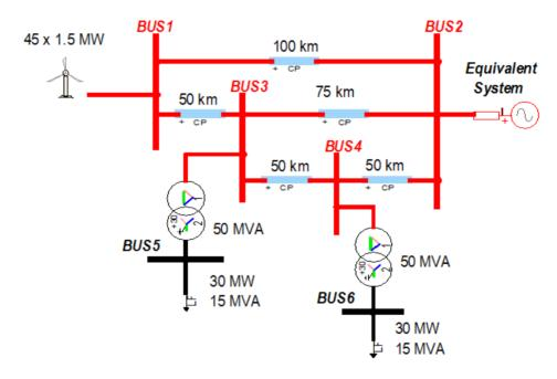
Figure 46 120 kV, 60 Hz test system
