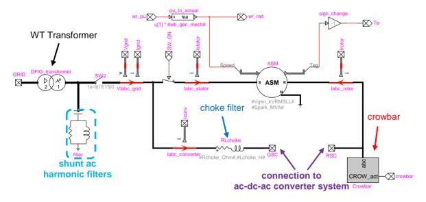
Figure 36 EMTP diagram of DFIG "WT Electrical System" block
