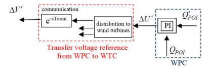
Figure 5 Reactive power control at POI (Q-control function)
