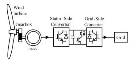
Figure 6 FSC wind turbine configuration
