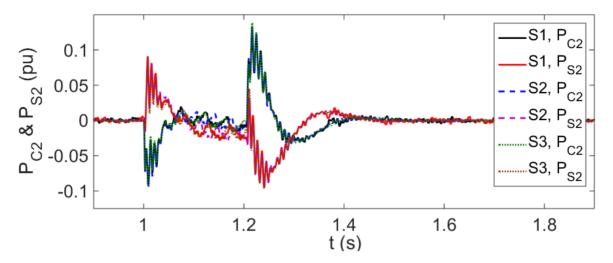
Figure 67  $P_{C2}$  and  $P_{S2}$  of aggregated FSC WT in IEEE 39 bus system simulation
