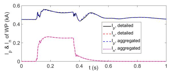
Figure 80 Positive and negative sequence currents at POI, Wind Park with DFIG WTs
