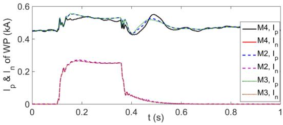
Figure 65 In and Ip of DFIG WT based WP in scenarios M2 - M4
