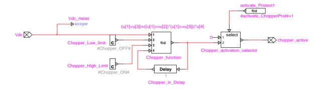
Figure 33 dc overvoltage protection block
