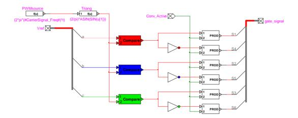
Figure 15 PWM control block
