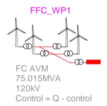
Figure 11 FSC based wind park device, mask parameters shown in Figure 12
