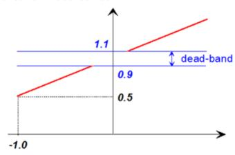
Figure 27 Wind turbine reactive output current during voltage disturbances [13].
