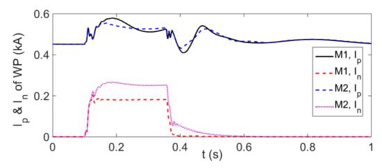
Figure 56 In and Ip of DFIG WT based WP in scenarios M1 and M2
