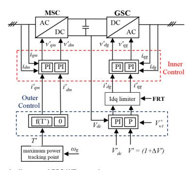
Figure 8 Schematic diagram of FSC WT control
