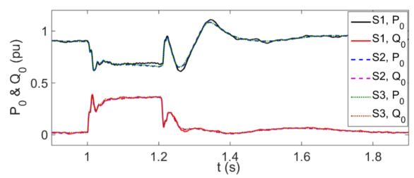
Figure 71 P<sub>0</sub> and Q<sub>0</sub> of aggregated DFIG WT in IEEE 39 bus system simulation
