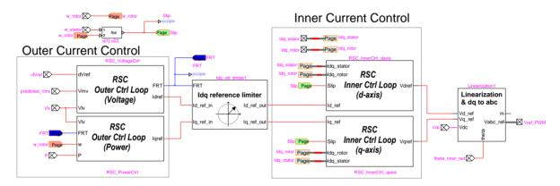
Figure 39 EMTP diagram of DFIG "Rotor Control" block
