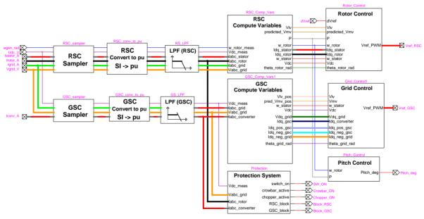
Figure 37 EMTP diagram of DFIG "WT Control System" block
