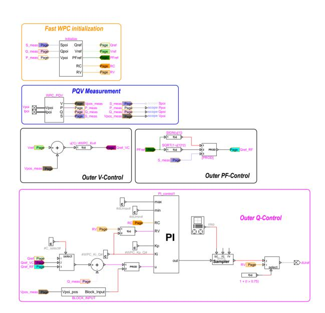
Figure 19 EMTP diagram of "WP Control System" block
