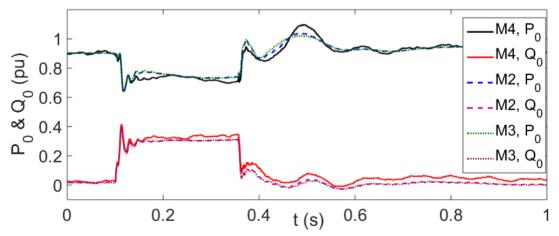
Figure 64 P<sub>0</sub> and Q<sub>0</sub> of aggregated DFIG WT in scenarios M2 - M4
