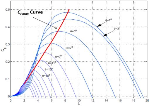
Figure 2 Wind power C<sub>p</sub> curves
