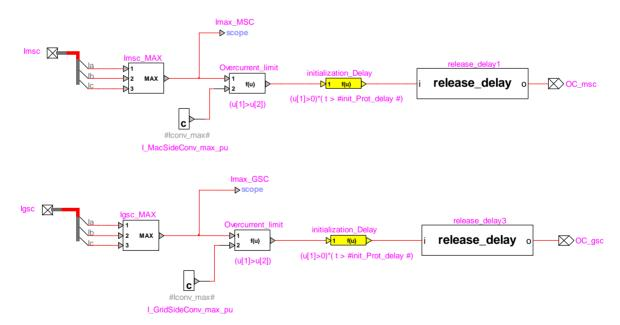
Figure 34 Overcurrent protection block
