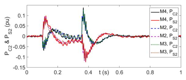
Figure 60 P<sub>C2</sub> and P<sub>S2</sub> of aggregated FSC WT in scenarios M2 - M4
