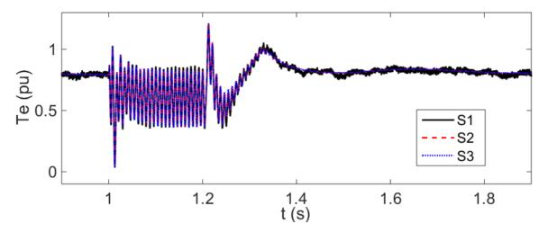
Figure 70 IG electromagnetic torque in IEEE 39 bus system simulation
