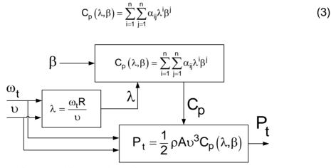
Figure 3 Wind turbine model for aerodynamics
