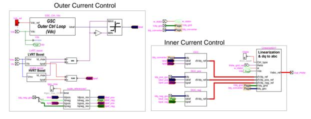
Figure 42 EMTP diagram of DFIG "Grid Control" block
