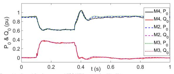
Figure 61 P₀ and Q₀ of aggregated FSC WT in scenarios M2 - M4
