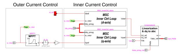
Figure 24 EMTP diagram of FSC "PMSG Control" block
