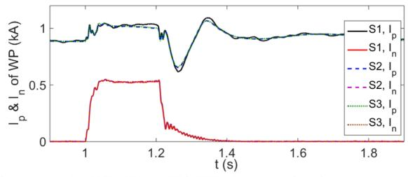
Figure 72  $I_n$  and  $I_p$  of DFIG WT based WP in IEEE 39 bus system simulation
