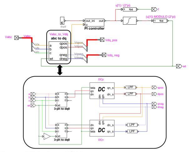
Figure 23 EMTP-RV diagram of DSRF PLL
