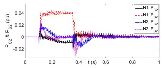
Figure 50 P<sub>C2</sub> and P<sub>S2</sub> of aggregated FSC WT in scenarios N1 and N2
