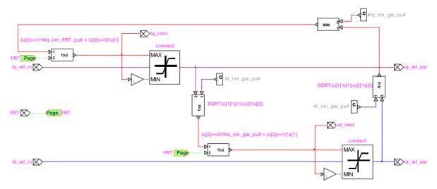
Figure 28 EMTP diagram of "Idq reference limiter" block
