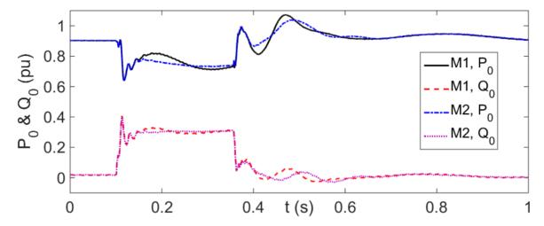
Figure 58 P and Q of aggregated DFIG WT in scenarios N1 and N2
