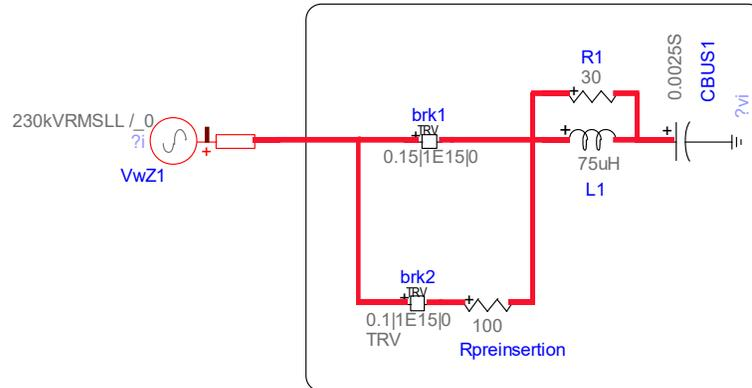
Figure 3-3: Master/Slave between Breakers for TRV
