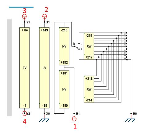
Transformer wide-band model: Damping Function (DF)
