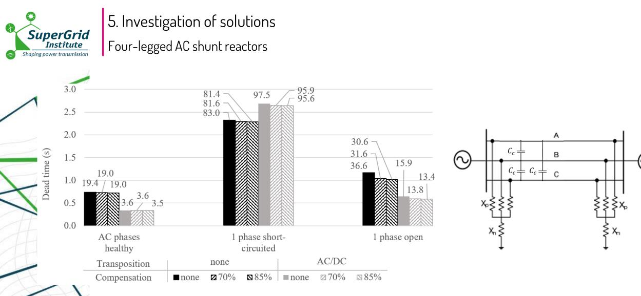
The presence of the four-legged AC shunt reactors does not worsen the situation regarding the SAC and dead time
