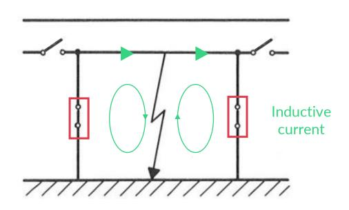
The association of line transposition and HSES is to be avoided because it could even lead to permanent faults
