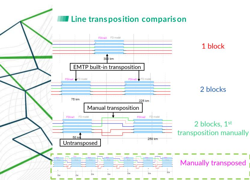
Time domain simulations are not suited for line transposition with several line blocs.
