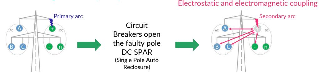
The secondary arc must be extinguished before the line is closed.
